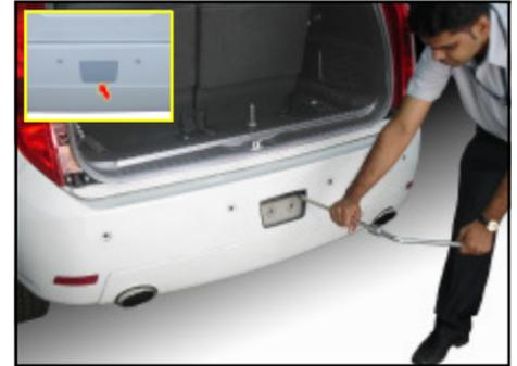
4. Rotate the handle anti-clockwise to lower the spare wheel till it rests on the ground.
