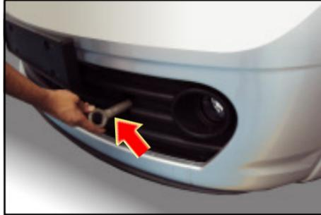
*Tow Hook Attachment Location at Front*
