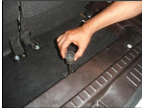
2. Remove the window cover provided on the rear bumper to access the spare wheel bracket.
